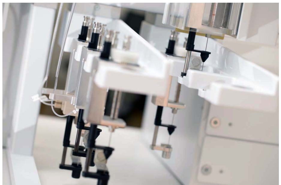
图1: Robotic Tool Change, Park Station
